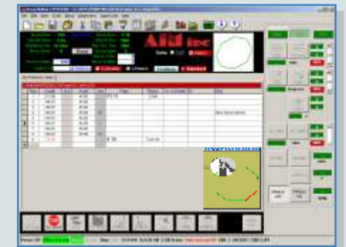
Simple Programming Interface. SmartEditor® helps figure out machine movements. User only needs to add feed length, bend angle, radius size & tool configuration.
