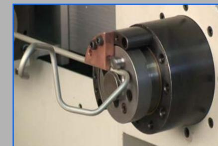
Simple Tooling for Wire or Tube Configuration
